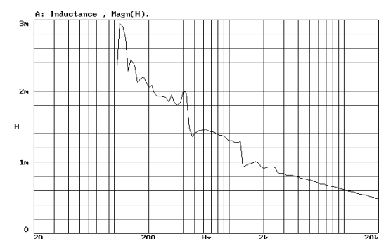
VOICE COIL INDUCTANCE CURVE
